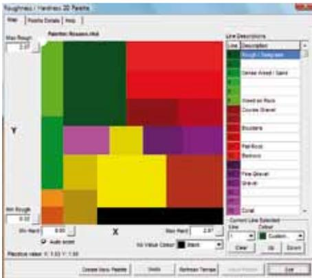
Shown below is the RoxAnn RH 2D palette installed with Piscatus<sup>3D</sup>. The Y values represent Roughness and the X values represent Hardness. Different combinations of RH data represent different seafloor types and each type is assigned a colour and a description.
