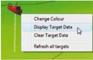
To display information about an ARPA target right click on the ARPA target inside the 3D, the menu shown to the left will be displayed. Select the option 'Display Target Data' from the menu. Only one target can display information.
