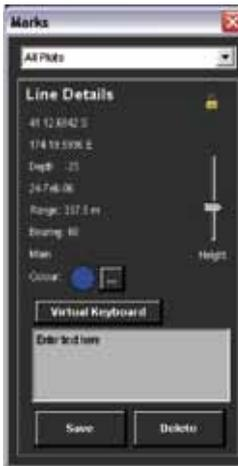
6. After you have created a new line you will notice an information panel appears, as shown on the left. This area details the start co-ordinates of the line, when it was created, what plot it is part of and what depth it is placed at. There is also a text box where you can write a description or add notes related to the line.
