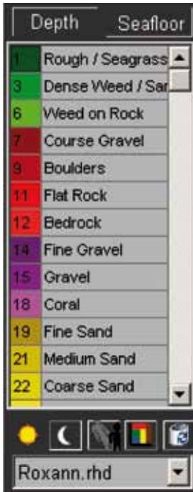
When the 'Seafl oor' option is selected and RH data is being display in the 3D, the colours used on the 3D terrain refer to the selected 2D palette. In the example shown on the left the RoxAnn 2D palette is selected.
